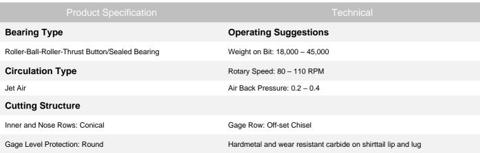
Based on the IADC Bit Classification System located in the IADC Drilling Manual, 11th Ed. – Redesigned, 2007
